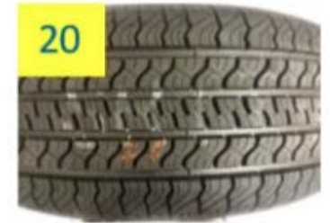
SRTT - Standard Reference Test Tire
